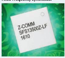
The SFS13500Z-LF is a single frequency signal source that is pre-programmed to operate at 13.5 GHz. This fixed frequency PLL has a typical phase noise of -80 dBc/Hz at 10 kHz offset with a reference spur suppression of -65 dBc. It is designed to operate over the temperature range of -40° to +85°C while delivering 0 dBm of output power into a 50 ohm load and is available in a package measuring  $1^{\rm w} \times 1^{\rm w} \times 0.22^{\rm w}$ .
