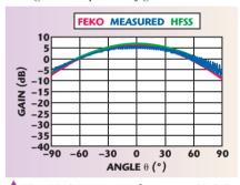
Fig. 14 Comparison of gains at 1.25 GHz.
