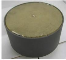
Fig. 9 Two-arm spiral antenna prototype with helices and wraparound absorber.
