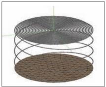
▲ Fig. 6 Spiral antenna with helices connecting the spiral to the ground plane.
