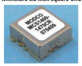
Modco announces its MCS Series CRO's. Low Vcc of 3.3V and current consumption of 13ma and makes it ideal for battery powered applications. Model Number MCS1400-1470CR tunes 1400-1470MHz with a Vt of 0.3-2.7V It provides 0dBm output power. Phase Noise is -110dBc @ 10kHz Pushing is 0.2MHz per volt and Pulling is 0.9MHz. Many models are available.
