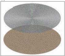
Fig. 2 Meshed FEKO model of benchmark antenna
